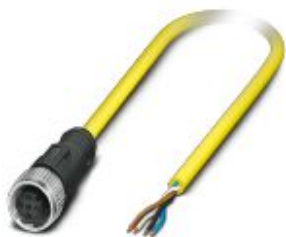
Sensor/actuator cable, 4-position, PVC, yellow, free cable end, on Socket straight M12, coding: A, cable length: 20 m
