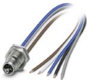
Flush-type connector, Power, 5-position, Plug, M12, L - Power, Rear mounting, M16 x 1.5, Individual wires, cable length: 0.2 m, 2.50 mm 2 , PEX litz wire
