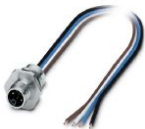
Flush-type connector, Power, 4-position, Plug, M12, L - Power, Front mounting, M16 x 1.5, Individual wires, cable length: 0.2 m, 2.50 mm 2 , PEX litz wire
