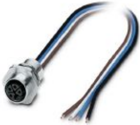
Flush-type connector, Power, 4-position, Socket, M12, L - Power, Front mounting, M16 x 1.5, Individual wires, cable length: 0.2 m, 2.50 mm 2 , PEX litz wire
