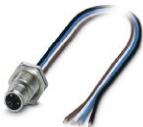
Flush-type connector, Power, 4-position, Plug, M12, L - Power, Rear mounting, M16 x 1.5, Individual wires, cable length: 0.2 m, 2.50 mm 2 , PEX litz wire
