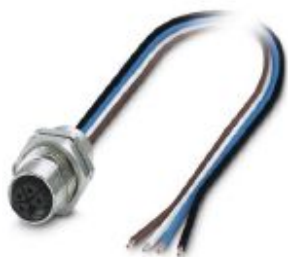
Flush-type connector, Power, 4-position, Socket, M12, L - Power, Rear mounting, M16 x 1.5, Individual wires, cable length: 0.2 m, 2.50 mm 2 , PEX litz wire
