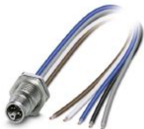
Flush-type connector, Power, 5-position, Plug, M12, L - Power, Rear mounting, M16 x 1.5, Individual wires, cable length: 0.2 m, 1.31 mm 2 , UL/cUL stranded hook-up wire
