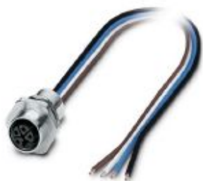
Flush-type connector, Power, 4-position, Socket, M12, L - Power, Front mounting, M16 x 1.5, Individual wires, cable length: 0.2 m, 1.31 mm 2 , UL/cUL stranded hook-up wire
