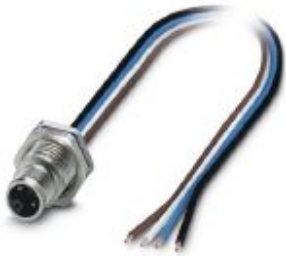
Flush-type connector, Power, 4-position, Plug, M12, L - Power, Rear mounting, M16 x 1.5, Individual wires, cable length: 0.2 m, 1.31 mm 2 , UL/cUL stranded hook-up wire
