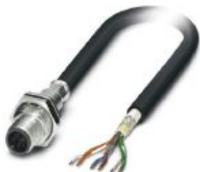
Bus system flush-type plug, VARAN, 6-pos., M12, shielded, rear/screw mounting with M16 thread, with 1 m bus cable
