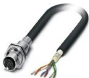
Bus system flush-type socket, VARAN, 6-pos., M12, shielded, rear/screw mounting with M16 thread, with 5 m bus cable
