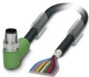
Sensor/actuator cable, 12-position, PUR/PVC, black RAL 9005, shielded, Plug angled M12 SPEEDCON, coding: A, on free cable end, cable length: 3 m
