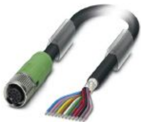
Sensor/actuator cable, 12-position, PUR/PVC, black RAL 9005, shielded, free cable end, on Socket straight M12 SPEEDCON, coding: A, cable length: 3 m
