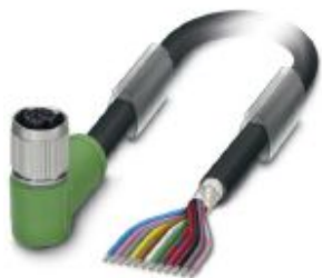
Sensor/actuator cable, 12-position, PUR/PVC, black RAL 9005, shielded, free cable end, on Socket angled M12 SPEEDCON, coding: A, cable length: 5 m
