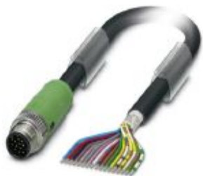
Sensor/actuator cable, 17-position, PUR/PVC, black RAL 9005, shielded, Plug straight M12 SPEEDCON, coding: A, on free cable end, cable length: 3 m
