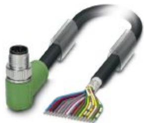
Sensor/actuator cable, 17-position, PUR/PVC, black RAL 9005, shielded, Plug angled M12 SPEEDCON, coding: A, on free cable end, cable length: 1.5 m
