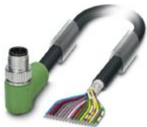
Sensor/actuator cable, 17-position, PUR/PVC, black RAL 9005, shielded, Plug angled M12 SPEEDCON, coding: A, on free cable end, cable length: 5 m
