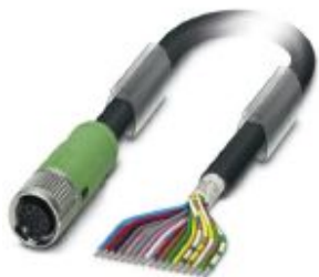
Sensor/actuator cable, 17-position, PUR/PVC, black RAL 9005, shielded, free cable end, on Socket straight M12 SPEEDCON, coding: A, cable length: 5 m
