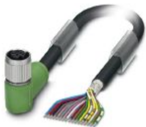
Sensor/actuator cable, 17-position, PUR/PVC, black RAL 9005, shielded, free cable end, on Socket angled M12 SPEEDCON, coding: A, cable length: 5 m
