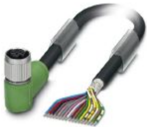
Sensor/actuator cable, 17-position, PUR/PVC, black RAL 9005, shielded, free cable end, on Socket angled M12 SPEEDCON, coding: A, cable length: 10 m
