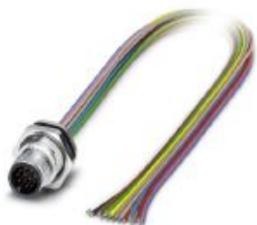
Sensor/actuator flush-type plug, 12-pos., M12 SPEEDCON, rear/screw mounting with Pg9 thread, with 0.5 m halogen-free TPE litz wire, 12 x 0.14 mm 2
