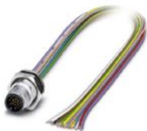
Sensor/actuator flush-type plug, 17-pos., M12 SPEEDCON, rear/screw mounting with Pg9 thread, with 0.5 m halogen-free TPE litz wire, 17 x 0.14 mm 2
