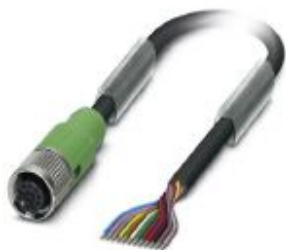
Sensor/actuator cable, 12-position, PUR halogen-free, black RAL 9005, free cable end, on Socket straight M12 SPEEDCON, coding: A, cable length: 3 m
