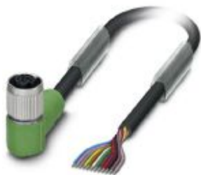
Sensor/actuator cable, 12-position, PUR halogen-free, black RAL 9005, free cable end, on Socket angled M12 SPEEDCON, coding: A, cable length: 10 m
