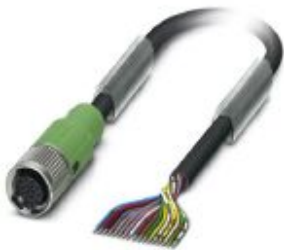
Sensor/actuator cable, 17-position, PUR halogen-free, black RAL 9005, free cable end, on Socket straight M12 SPEEDCON, coding: A, cable length: 3 m
