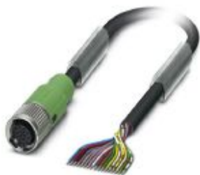
Sensor/actuator cable, 17-position, PUR halogen-free, black RAL 9005, free cable end, on Socket straight M12 SPEEDCON, coding: A, cable length: 10 m
