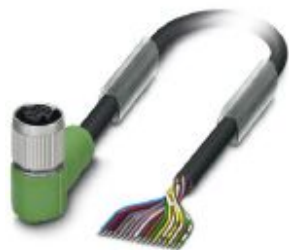
Sensor/actuator cable, 17-position, PUR halogen-free, black RAL 9005, free cable end, on Socket angled M12 SPEEDCON, coding: A, cable length: 5 m
