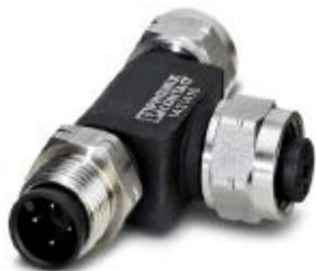
T distributor, FOUNDATION Fieldbus, FOUNDATION Fieldbus, 4-position, unshielded, Plug straight M12, coding: A, on Socket straight M12, coding: A and Socket straight M12, coding: A, Parallel distributor
