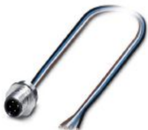
Bus system flush-type connector, FOUNDATION Fieldbus, plug, 4-pos., M12, A-coded, front/screw mounting with Pg9 thread, with 0.5 m TPE litz wire, 3 x 0.34 mm 2 , stainless steel version
