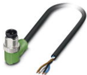
Sensor/actuator cable, 4-position, PVC, black RAL 9005, Plug angled M12, A - standard, on free cable end, cable length: 10 m
