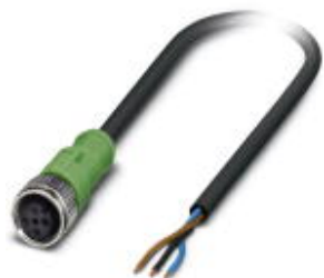
Sensor/actuator cable, 3-position, PVC, black RAL 9005, free cable end, on Socket straight M12, A-coded, cable length: 2 m
