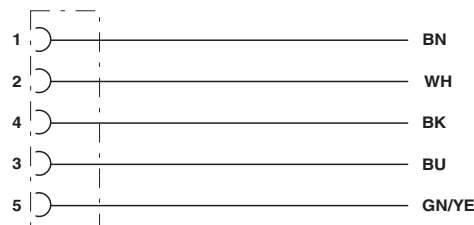
Contact assignment of the M12 sockets
