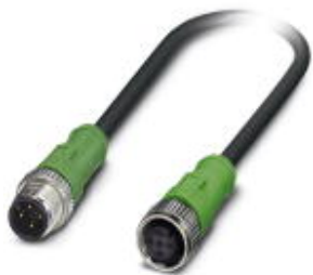
Sensor/actuator cable, 4-position, PVC, black RAL 9005, Plug straight M12, A - standard, on Socket straight M12, A - standard, cable length: 0.6 m
