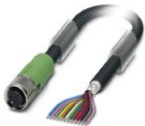
Sensor/actuator cable, 12-position, PUR/PVC, black RAL 9005, shielded, free cable end, on Socket straight M12 SPEEDCON, coding: A, cable length: 1 m
