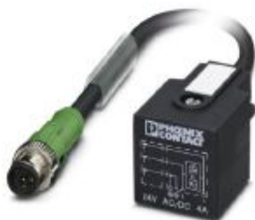
Sensor/actuator cable, 3-position, PUR halogen-free, black-gray RAL 7021, Plug straight M12 SPEEDCON, coding: A, on Valve connector A, with 1 LED, connected with Z diode, cable length: 3 m
