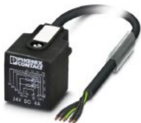
Sensor/actuator cable, 5-position, PUR halogen-free, black-gray RAL 7021, free cable end, on Valve connector AD (pressure switch), with 2 LEDs, cable length: 10 m
