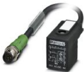
Sensor/actuator cable, 3-position, PUR halogen-free, black-gray RAL 7021, Plug straight M12 SPEEDCON, coding: A, on Valve connector BI (11 mm), with 1 LED, connected with Z diode, cable length: 0.6 m
