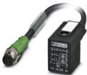
Sensor/actuator cable, 3-position, PUR halogen-free, black-gray RAL 7021, Plug straight M12 SPEEDCON, coding: A, on Valve connector BI (11 mm), with 1 LED, connected with Z diode, cable length: 3 m
