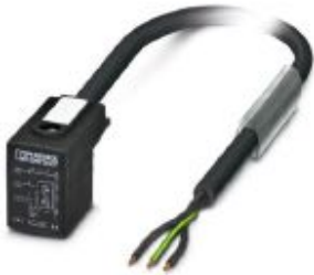
Sensor/actuator cable, 3-position, PUR halogen-free, black-gray RAL 7021, free cable end, on Valve connector BI (11 mm), with 1 LED, connected with Z diode, cable length: 3 m
