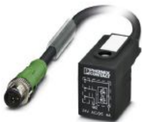
Sensor/actuator cable, 3-position, PUR halogen-free, black-gray RAL 7021, Plug straight M12 SPEEDCON, coding: A, on Valve connector B (10 mm), with 1 LED, connected with Z diode, cable length: 1.5 m
