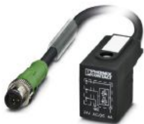
Sensor/actuator cable, 3-position, PUR halogen-free, black-gray RAL 7021, Plug straight M12 SPEEDCON, coding: A, on Valve connector B (10 mm), with 1 LED, connected with Z diode, cable length: 3 m
