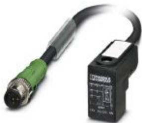
Sensor/actuator cable, 3-position, PUR halogen-free, black-gray RAL 7021, Plug straight M12 SPEEDCON, coding: A, on Valve connector C (8 mm), with 1 LED, connected with Z diode, cable length: 1.5 m
