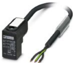
Sensor/actuator cable, 3-position, PUR halogen-free, black-gray RAL 7021, free cable end, on Valve connector CI (9.4 mm), with 1 LED, connected with Z diode, cable length: 10 m
