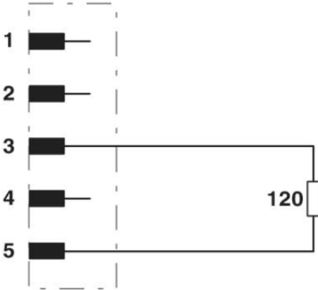
Internal wiring of connections
