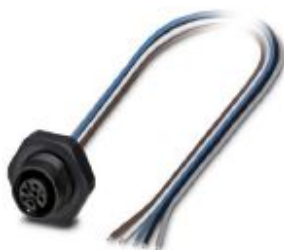
Sensor/Actuator flush-type connector, socket, 5-pos., M12, A-coded, rear/screw mounting with Pg9 thread, with 0.5 m TPE litz wire, 5 x 0.25 mm 2 , plastic version
