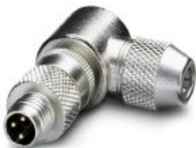
Connector, Universal, 3-position, shielded, Plug angled M8, Coding: A, Solder connection, knurl material: Nickel-plated brass, external cable diameter 3.5 mm ... 5 mm
