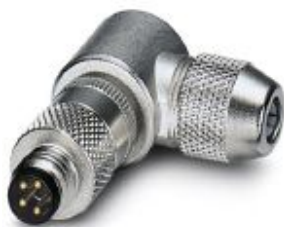
Connector, Universal, 4-position, shielded, Plug angled M8, Coding: A, Solder connection, knurl material: Nickel-plated brass, external cable diameter 3.5 mm ... 5 mm
