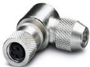
Connector, Universal, 4-position, shielded, Socket angled M8, Coding: A, Solder connection, knurl material: Nickel-plated brass, external cable diameter 3.5 mm ... 5 mm
