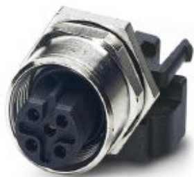
Sensor/actuator flush-type connector, socket, 5-pos., M12, shielded, B-coded, rear/screw mounting with M12 thread, with polarity protection, with straight solder connection
