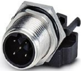
Sensor/actuator flush-type plug, 5-pos., M12, shielded, B-coded, rear/screw mounting with M12 thread, with straight solder connection
